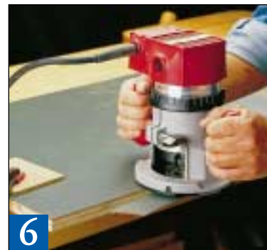
6 A flush-trim router bit, guided by a bearing, will shear the laminate off along the edges. Watch for voids in the substrate.
