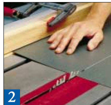
2 Laminates slide under most fences, so if you cut the material on the table saw, use a kerfed wood fence to guide the edge.
