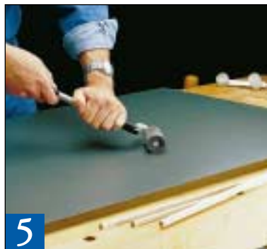
5 A J-roller helps ensure a strong cement bond. A double-wheel roller (in background) can do the edges after trimming.
